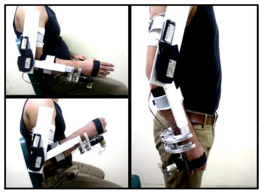
Figure 1: an example of an assistive device used to facilitate flexion and extension of the elbow joint (Image taken from Mohammedi, Zohoor and Khadem, 2016).
