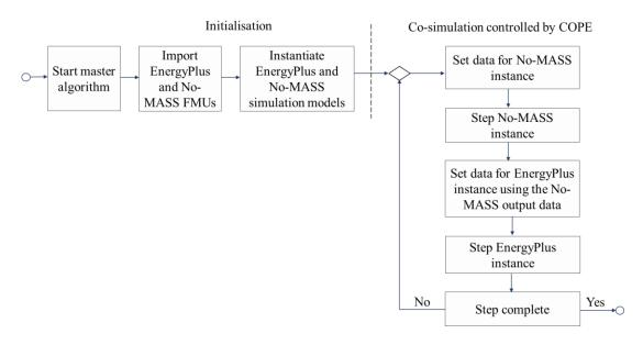
Figure 5.12: EnergyPlus and No-MASS single building co-simulation flow diagram (COPE approach)
