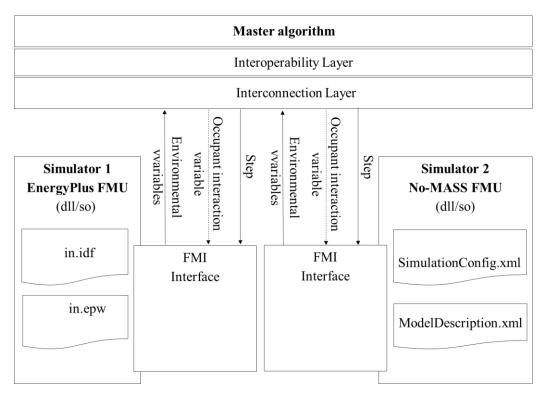
Figure 5.5: EnergyPlus and No-MASS orchestration diagram (COPE approach)
