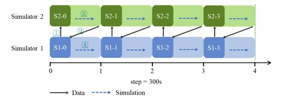
Figure 4.8: Gauss-Seidel type of weak coupling of two simulators
