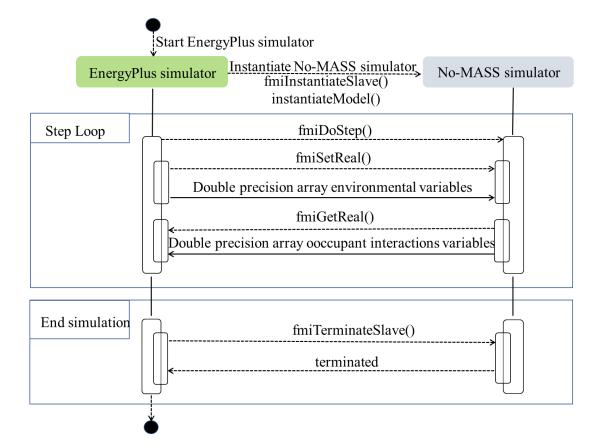
Figure 5.4: EnergyPlus and No-MASS co-simulation process (FMU import approach)
