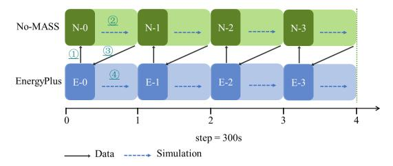
Figure 5.8: Data flow between EnergyPlus and No-MASS during co-simulation
