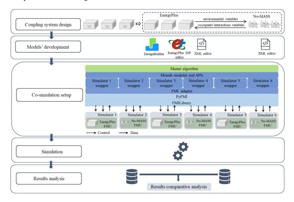
Figure 5.16: Multiple shoe box buildings co-simulation case study process
