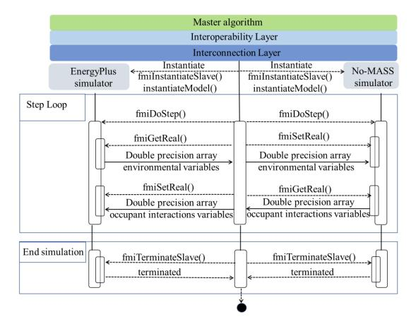
Figure 5.6: EnergyPlus and No-MASS co-simulation process (COPE approach)
