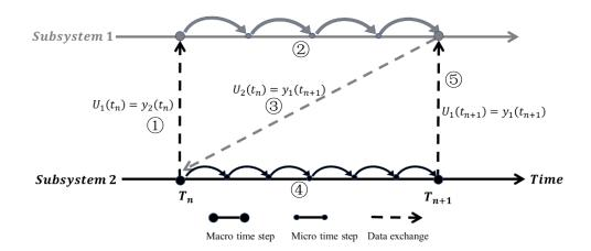
b) Gauss-Seidel type of weak coupling
