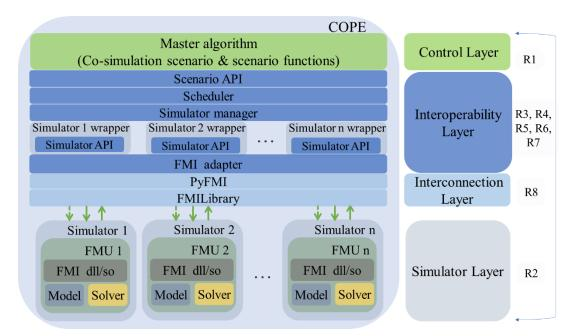
Figure 4.10: The co-simulation platform for Ecological-Urban - COPE
