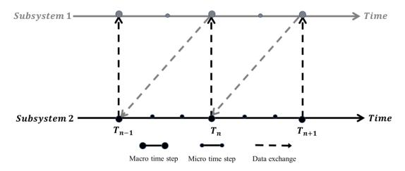
b) Weak coupling - sequential Gauss-Seidel type
