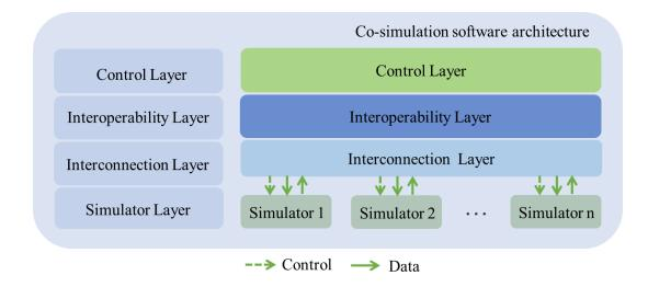
Figure 3.1: Conceptual architecture of the urban energy systems co-simulation
