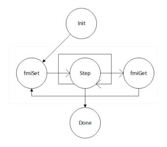
Figure 2.7: State Machine of Calling Sequence
