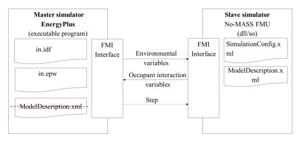
Figure 5.3: EnergyPlus and No-MASS orchestration diagram (FMU import approach - based on (Chapman, Siebers et al. 2018))
