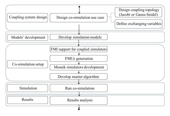
Figure 5.25: Process to conduct co-simulation based on the urban energy cosimulation platform
