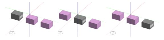
Figure 5.20: Three shoe box building DesignBuilder models
