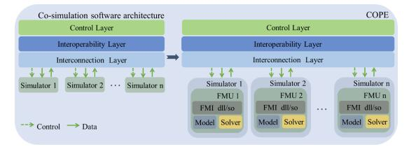
Figure 4.2: COPE – Detail of the simulator layer
