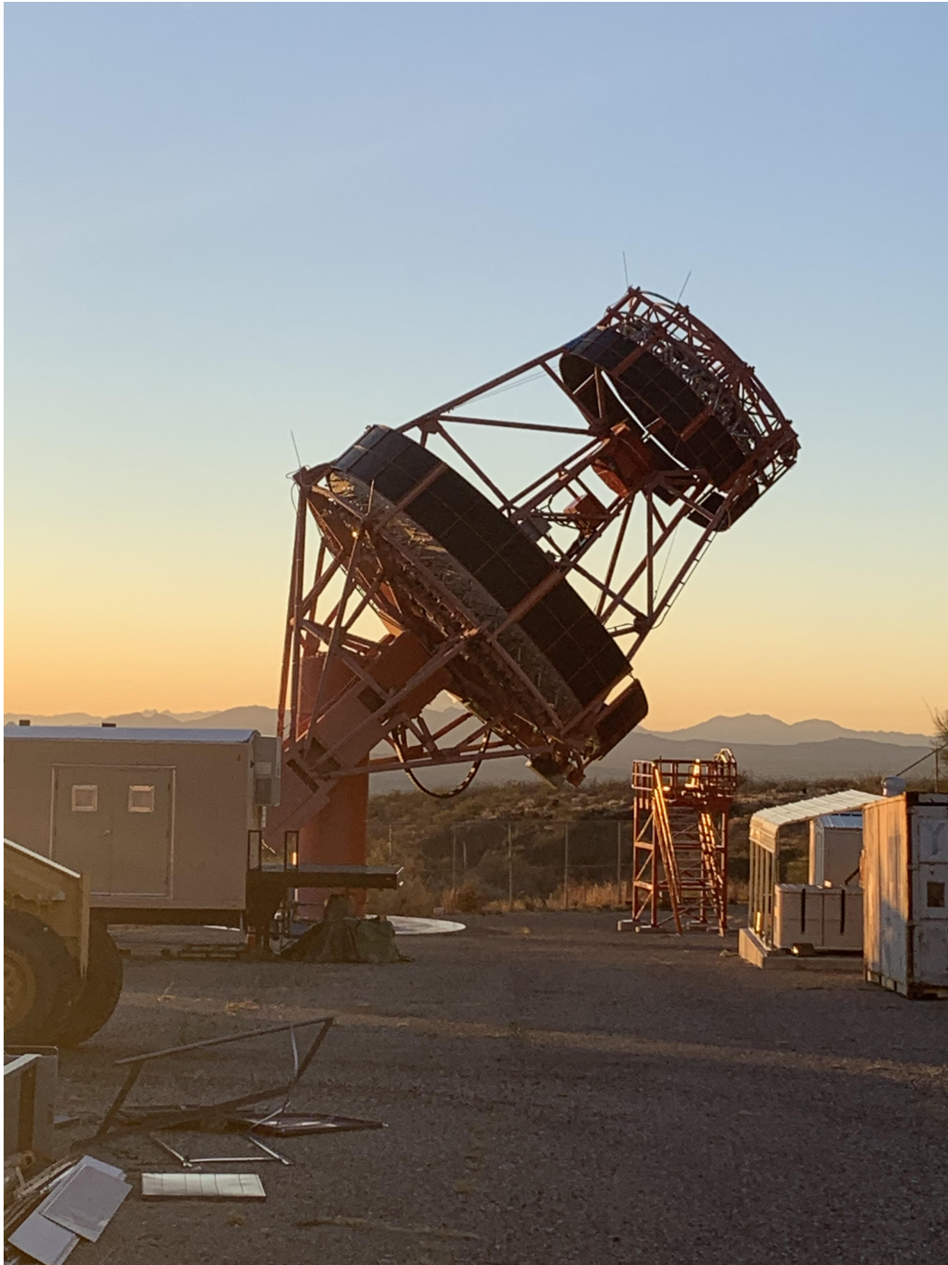
Figure 10.1: The prototype Schwarzschild-Couder dual mirror medium sized telescope, one of the two medium sized telescopes designed for CTA. The prototype SCT is located at the site of the VERITAS observatory, south of Tucson, Arizona.
