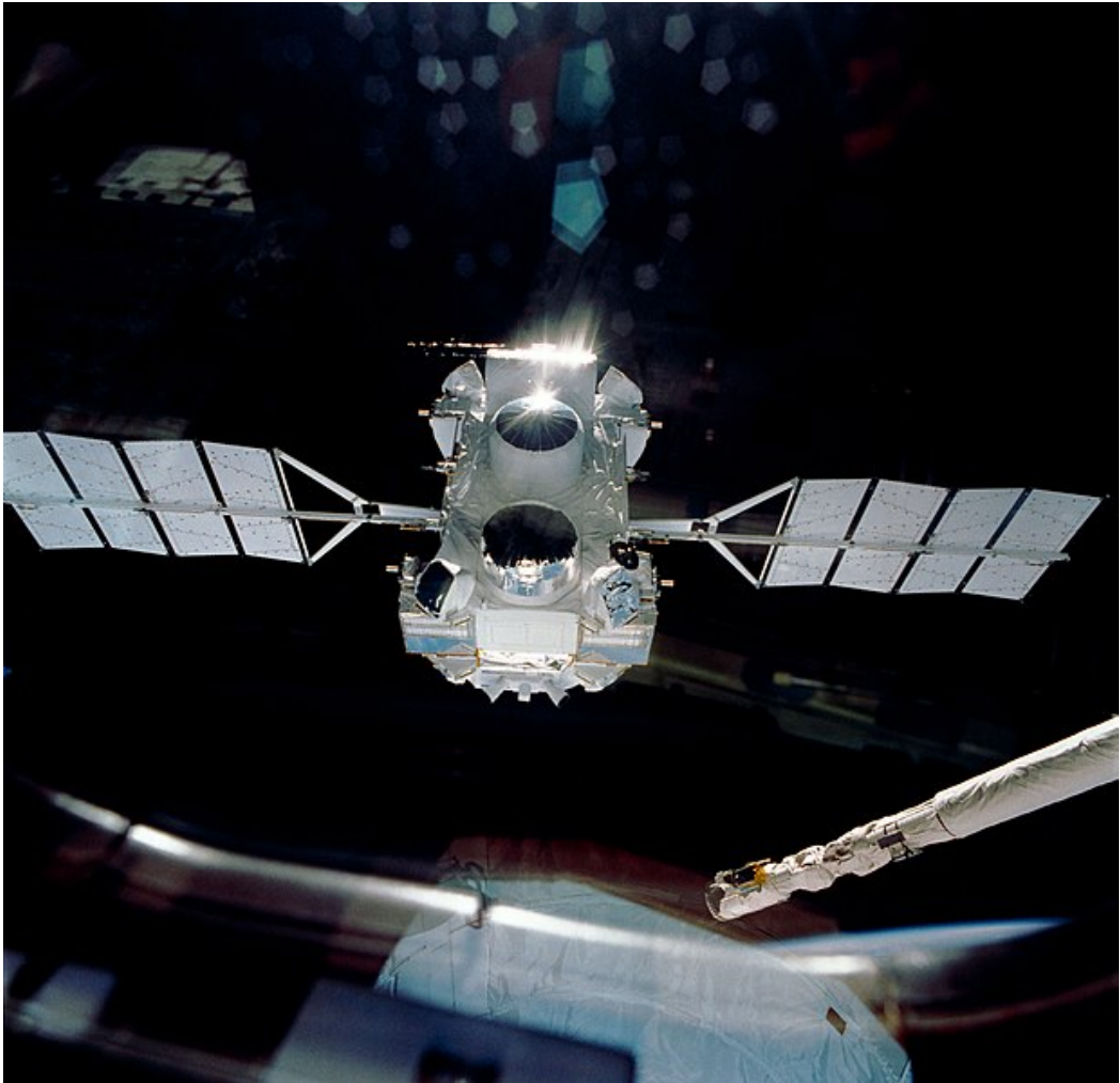
Figure 1.3: A photograph of the Compton Gamma-Ray Observatory as it is deployed from the space shuttle Atlantis in 1991. The space shuttle robotic arm is shown in the bottom of this image. Image credit: NASA.
