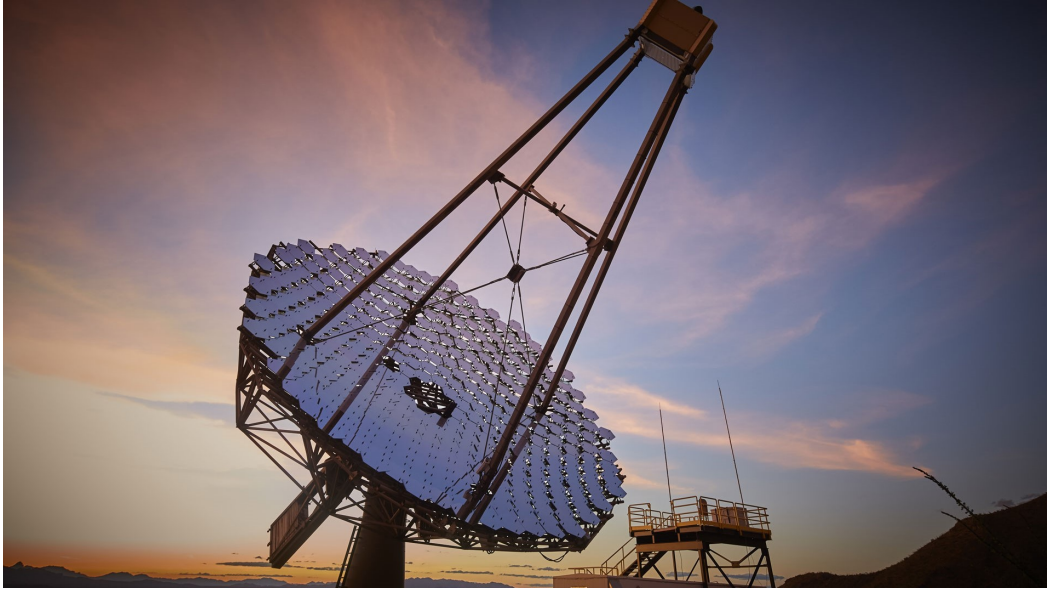
Figure 1.6: One of the four IACTs that make up the VERITAS array. Note the segmented mirror design, which allows individual panels to be removed for cleaning, maintenance and saves money compared to a larger single mirror reflector. The scaffolding platform in the background of the shot allows for maintenance to be performed on the telescope camera.
