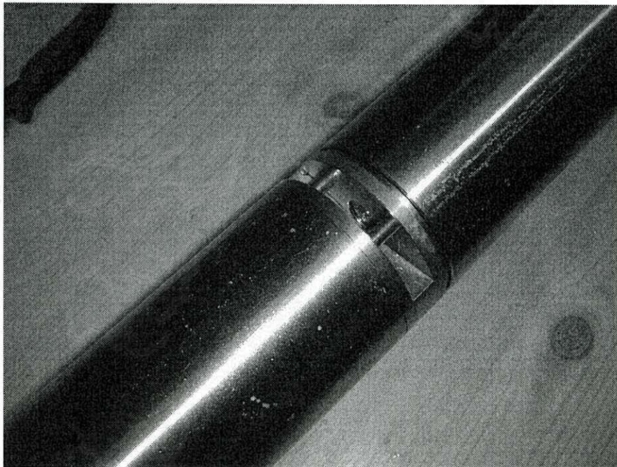
Figure 8.6: Close up of the sonde showing the opening for the windows where the measurement takes place.
