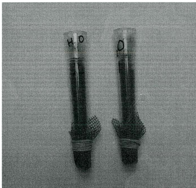
Figure II: The design of the leaching tubes used in Chapter 4.
