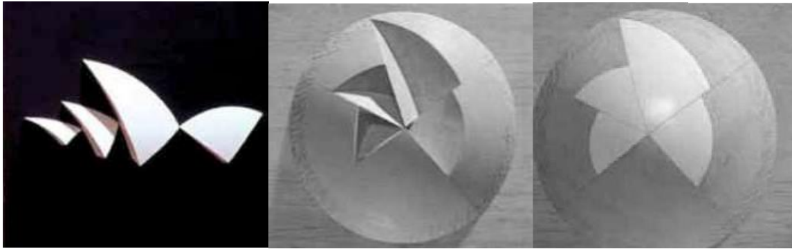
Figure 4: Sydney Opera House is define by the geometrical shape of the roof. The shells segment was taken from a single sphere. Each shell was made up of series of ribs formed by parallel lines Source: http://www.lilburnes.org/Students/Media2/Sydney
