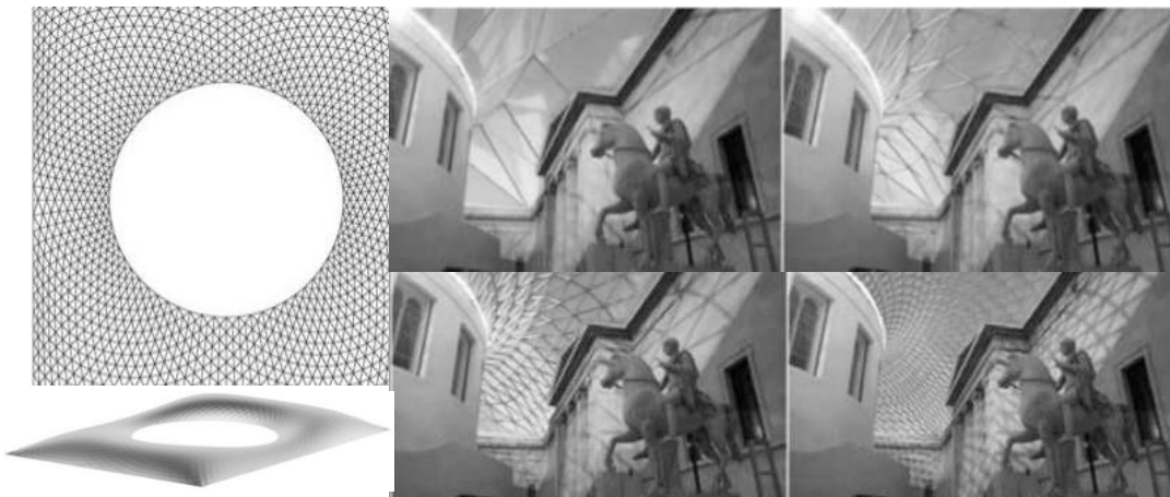
Figure 8: Steel grid, Faceted Surface and evolution of structural grid Source: The new mathematic of architecture
