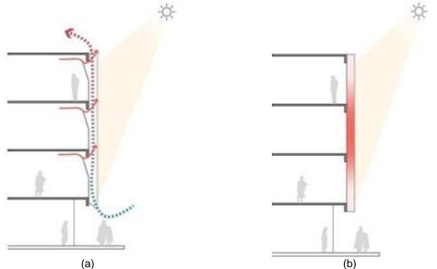
Figure 1. Comparison of heat mechanism in the DSF. (a) DSF in hot climate countries. (b) DSF in cold climate countries (Souza, 2022).
