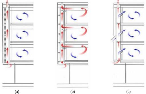
Figure 3. Type of DSF. (a) Buffer façade system (b) Extract-Air Façade System (c) Twin Face System (Boake, 2003).
