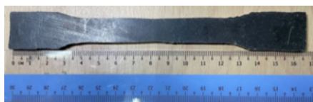
FIGURE 5. EPOXY GROUT B
