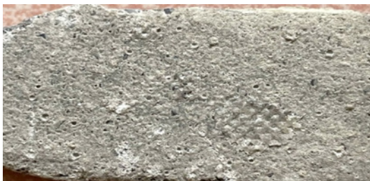
FIGURE 8. Surface of epoxy grout A after seawater adaption for 7 days
