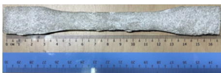
FIGURE 4. Epoxy grout A
