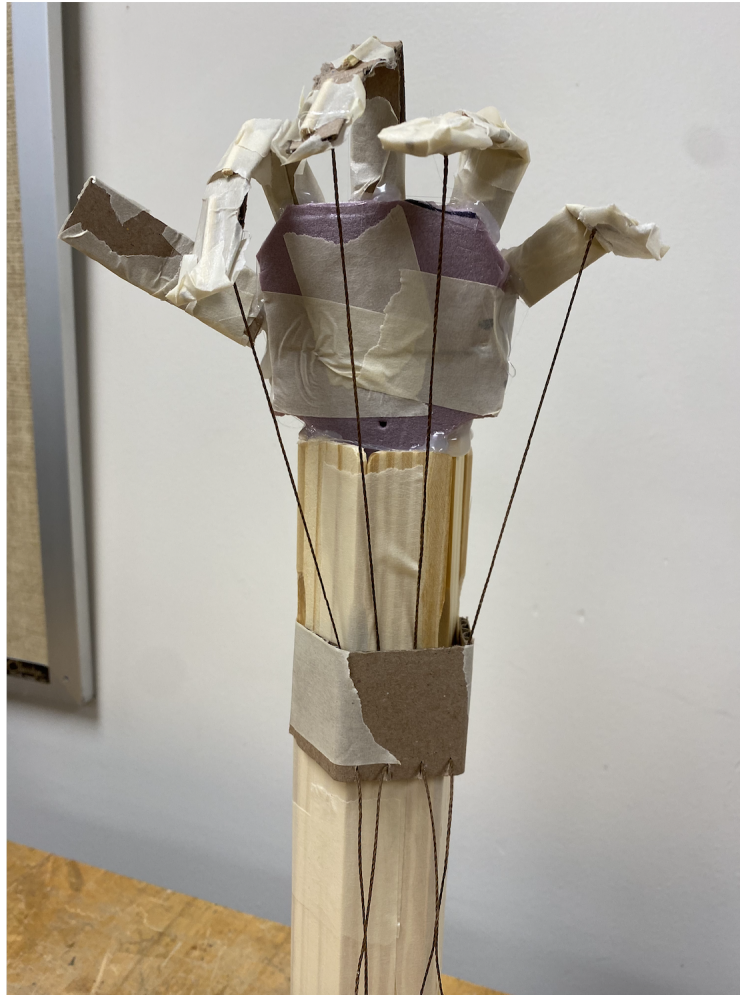
Figure 11: Mockup Prototype with string controlled fingers in a closed grip
