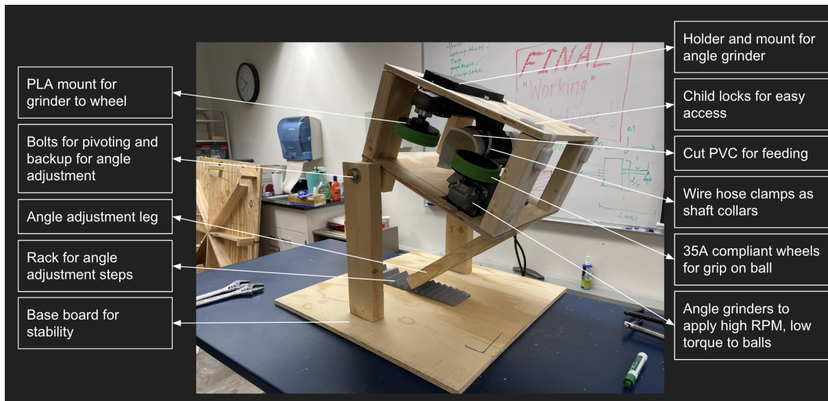
Figure 30: Components explanation of the final prototype.
