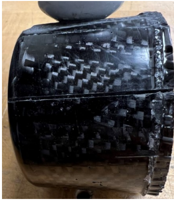
Figure 31: Carbon fiber- epoxy composite base
