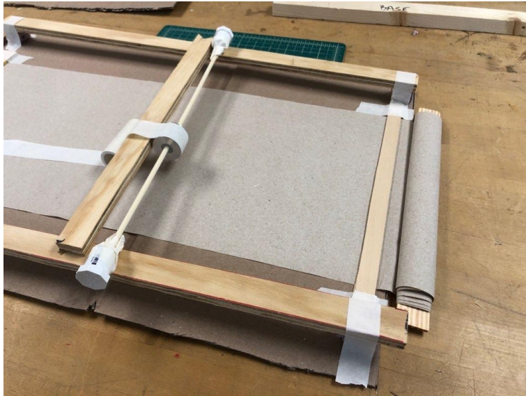
Figure 9: Close up of our storage and fabric dispensing tool
