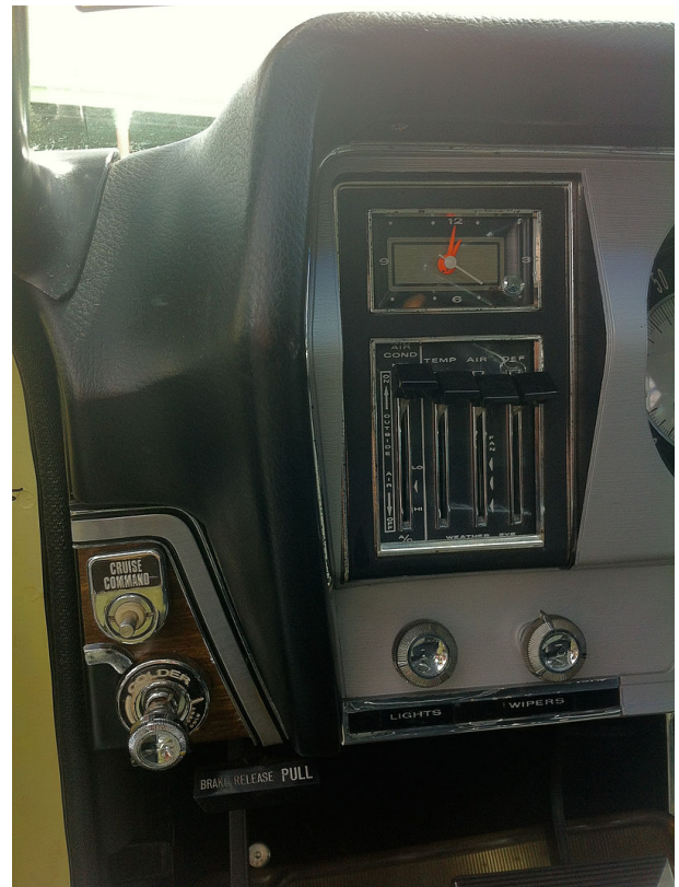
Figure 3: A button in the 1967 AMC Ambassador to engage and disengage cruise control (Source: American Cars, 1960-1972: Every Model, Year by Year)
