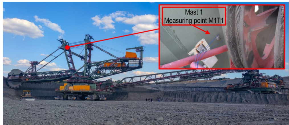
Figure 17. BWE SchRs 1600 during the measurements (conducted on 16 June 2021) and detail of the measurement point M1T1.
