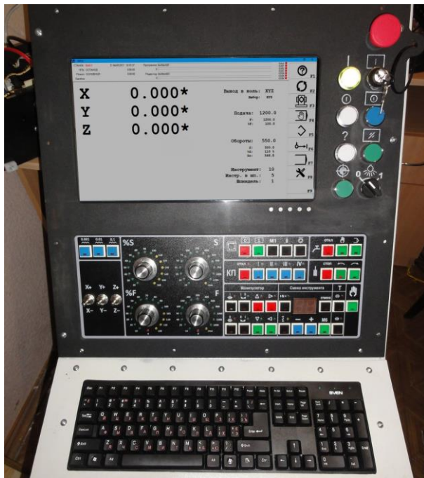
Figure 8: CNC control panel for modernization of the milling machine MA65SM30
