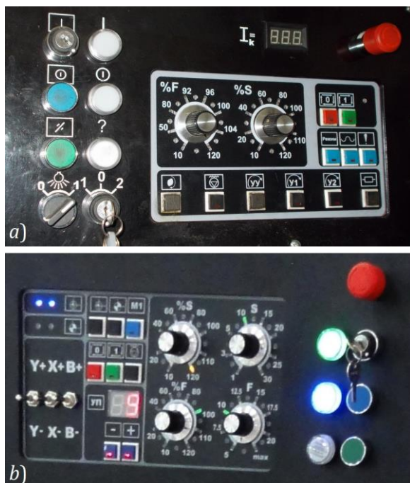
Figure 9: Operator panels for special CNC equipment: (a) operator panel for special machine for the continuous winding of fiberglass pipes; (b) operator panel for special for the bends winding machine [26]
