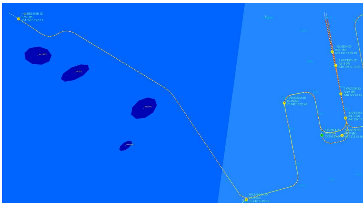
Figure 19. Route calculation for aircraft BEE156H approaching MXP from the northwest through a loose group of convective areas. If several convective cells occur as a group, the AMAN tries to guide aircraft around them as a whole. MXP traffic mix from 11 May 2019 with weather from 6 August 2019 and the RaNDeVIL nowcast model.
