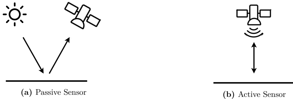
Figure 2.1. (a) Passive sensors detect the reflection of the sunlight from the object. (b) Active sensors have their own source of energy to illuminate the object.
