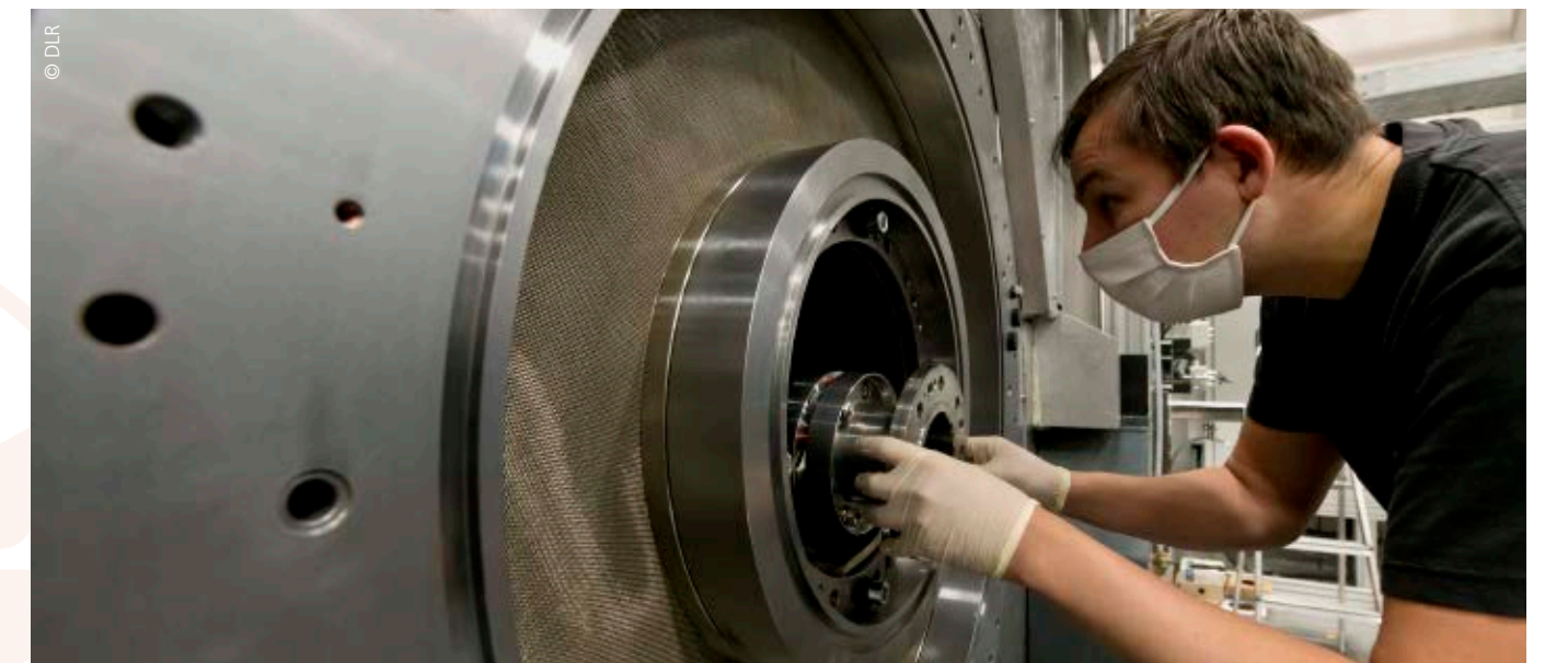
Installing the turbine shaft
