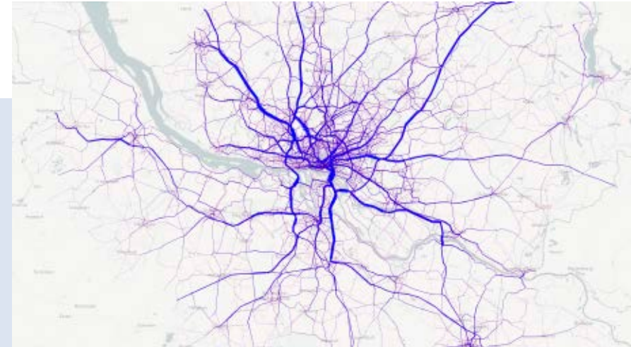
Automated shuttles on the road at the RealLab Hamburg (left). On the right, the MATSim traffic simulator shows the distribution of traffic in Hamburg. The thicker the road the more vehicles drove over it.
