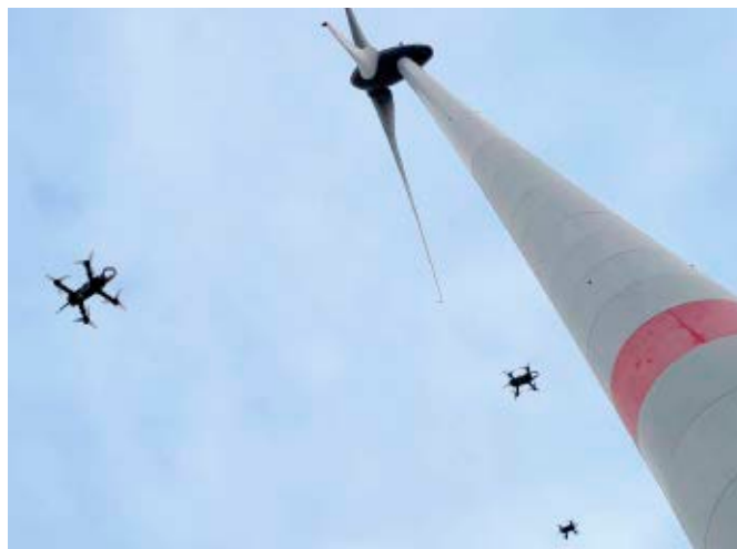
A first test to measure the flow phenomena with 20 drones has already been successful
