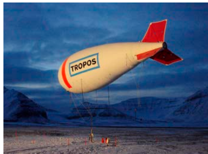
The tethered balloon BELUGA ready to be release in Ny Ålesund
