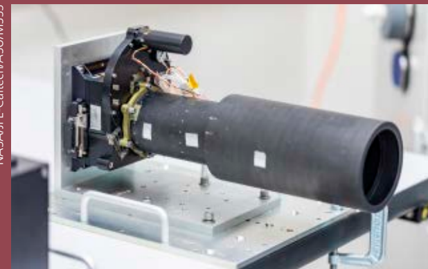
Psyche's high-resolution multispectral camera consists of a pair of identical cameras to image geology, topography and mineralogy. In addition, the cameras provide additional data for optical navigation.
