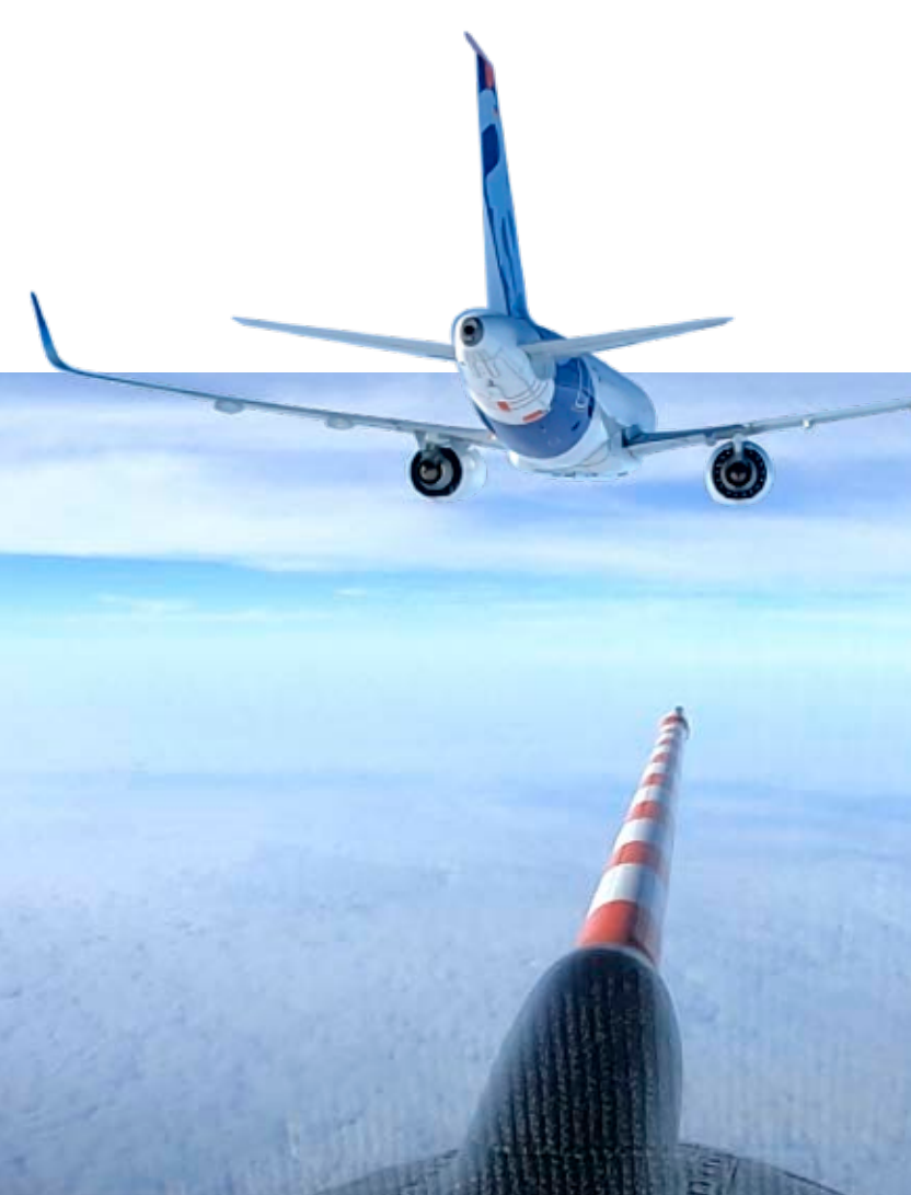
DLR's Falcon research aircraft measures emissions behind an Airbus A319neo
