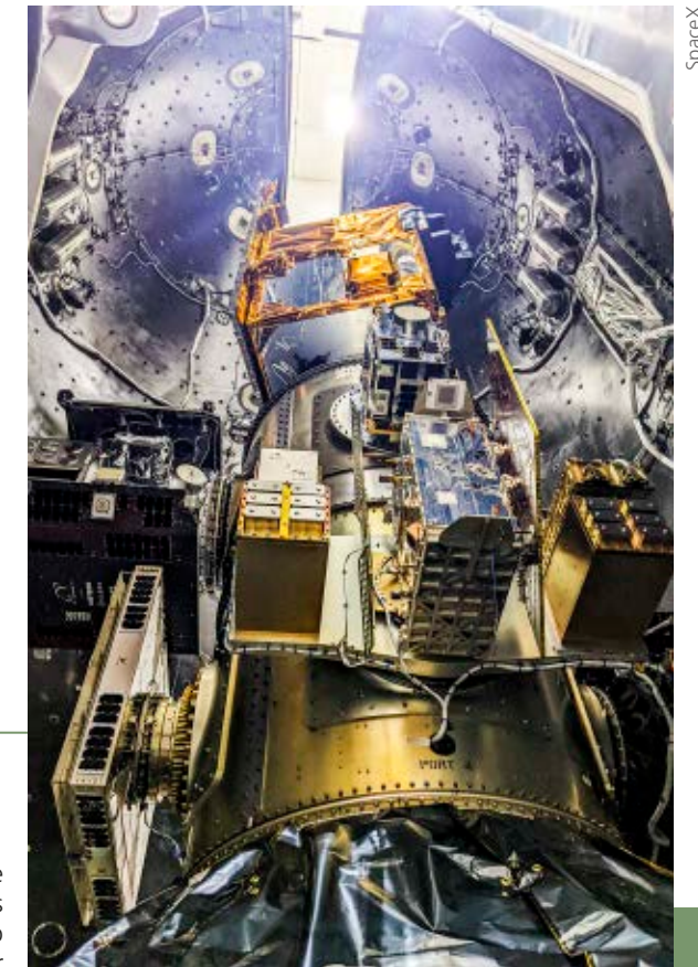
This photograph was taken shortly before the payload fairing for the Falcon 9 launcher was installed. It shows many of the 40 payload items, some of which are very small. EnMAP is at the top of the SpaceX Transporter-4 mission payload stack and is the largest satellite on board.
