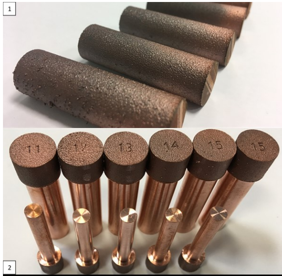
Figure 3.3. (1) Cylinders for LFA before machining to correct dimensions, showing discoloured surfaces due to heat treatment. (2) Larger diameter cylinders for LFA and smaller diameter cylinders for dilatometry after machining to correct diameter but before sectioning.
