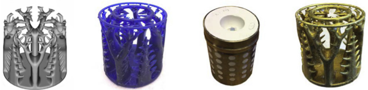
Figure 4.15. Investment casting of a topology optimised heat sink. The images shown (from left to right) show: the topology-optimised design, the castable resin pattern, the plaster mold and finally the metal heat sink. Reproduced from (Lei et al. 2018).
