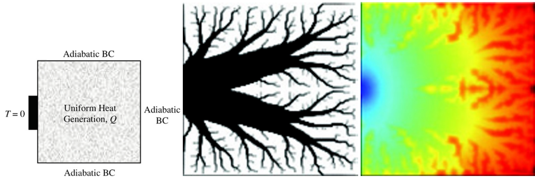
Figure 4.2. Left: Heat conduction topology optimisation domain and boundary conditions. Centre: topology optimised geometry with high conductivity material shown in black. Right: temperature distribution. Reproduced from (Ercan M Dede 2009).
