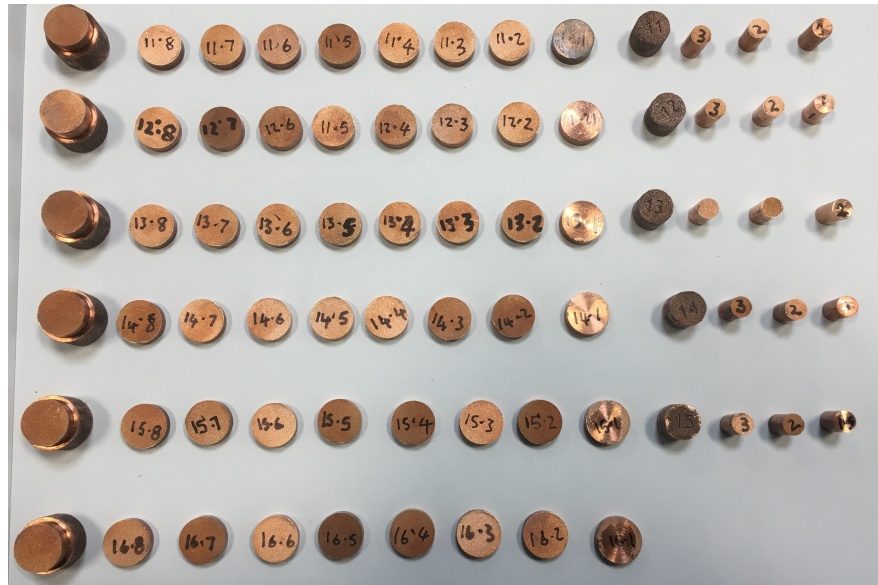
Figure 3.4. A selection of machined samples is displayed. The flatter samples on the left-hand side are for laser flash analysis and the small diameter cylinders on the right-hand side are for dilatometry. The image also includes the ends of the cylinders, which were not used for testing.
