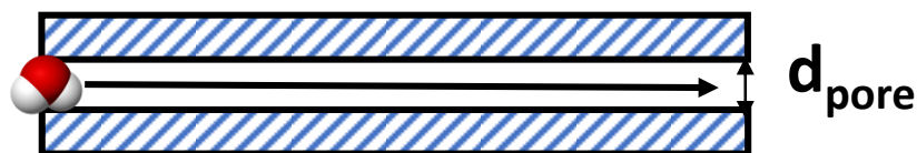
Figure 3.8. Configurational diffusion occurring within the pores of a porous medium. The pore diameter, d_{\text{pore}} , is approximately equal to the size of the diffusing species. The diffusion process will therefore be dominated by friction between the diffusing species and the pore wall.
