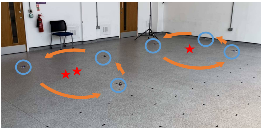
Fig. 8. A snapshot of the time-varying group formation mission during Experiment 2. The red stars mark the positions of three virtual targets.
