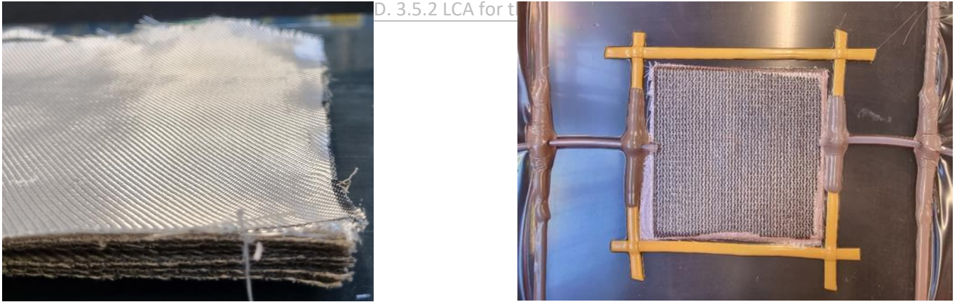
Figure F3: (left) the fibreglass peel ply above the laminate stack before bagging. (right) peel ply and flow medium laid over the fibres under vacuum conditions
