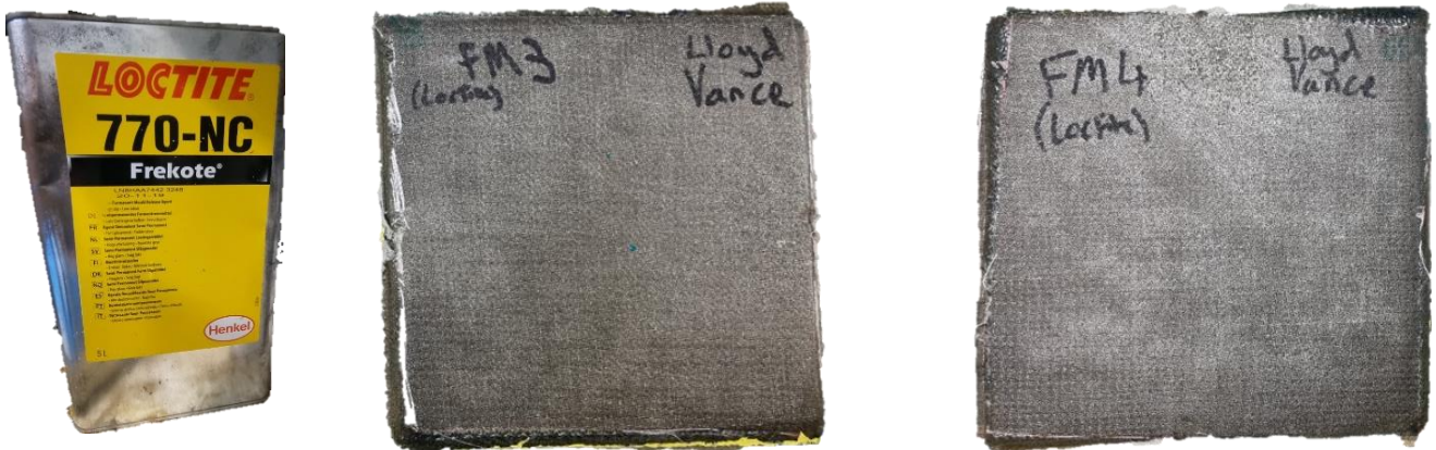
Figure F2: Loctite 770-NC label and plates FM3 and FM4.
