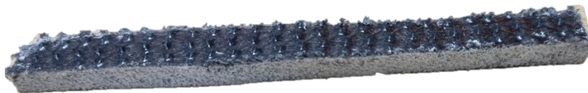
Figure F20: Image showing flow medium still bonded to test sample (Vance, 2022)
