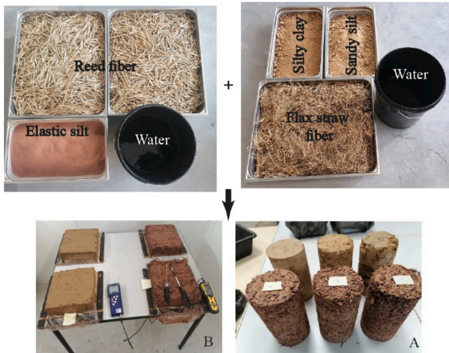
Fig. 6. Samples prepared for (A) water vapor permeability with porosity testing and (B) thermal conductivity measurement.
