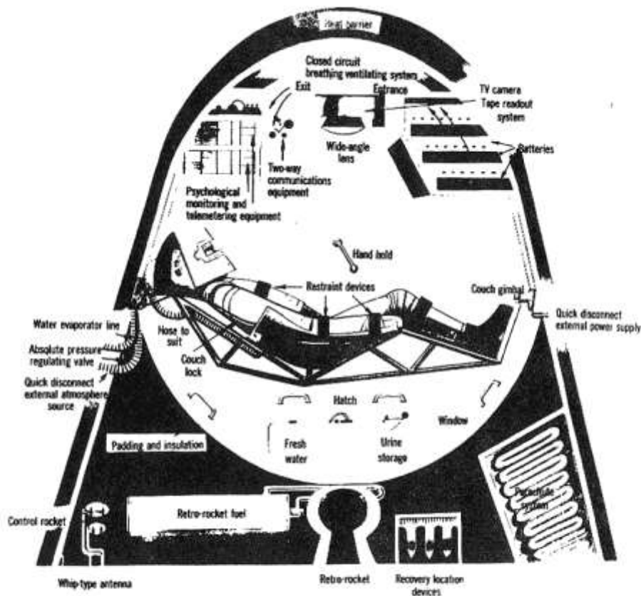
SKETCH shows how a passenger would look inside a spaceship. Comfort devices would be built into container for maximum reliability for both man and machine. Man, wearing spacesuit, reclines on couch for protection against gravity forces.
