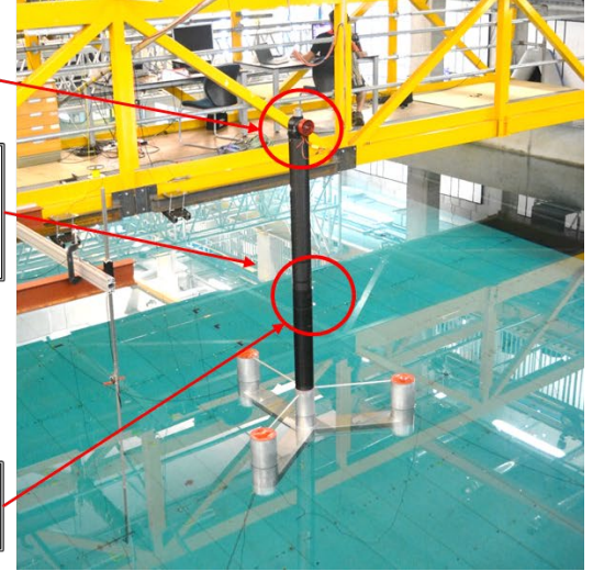
FIGURE 1: REAL-TIME HYBRID TESTING WORKFLOW (ADAPTED FROM [3]) (LEFT); 1:70 FROUDE-SCALED VOLTURNUS-PLATFORM IN THE COAST LABORATORY OCEAN BASIN AT THE UNIVERSITY OF PLYMOUTH, U.K. (RIGHT)
