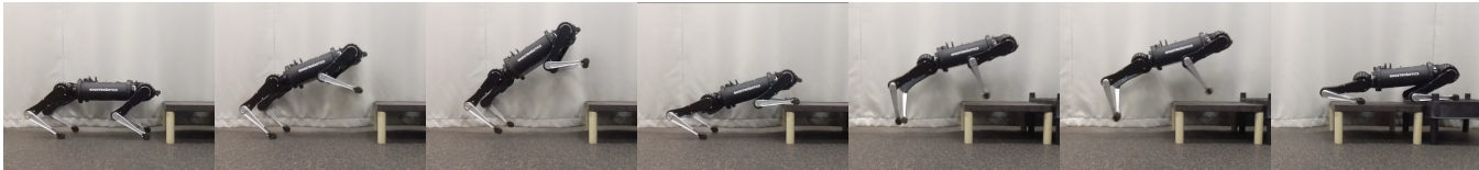
Fig. 6. Snapshots of Spirit performing the box-jump behavior from [22].
