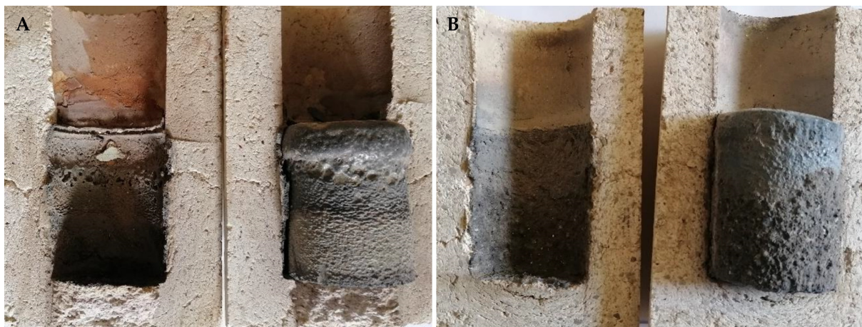
Figure 8. Degradation of refractory material MK 82 after high-temperature testing; (A) steel XT 720, (B) steel 11 523.
