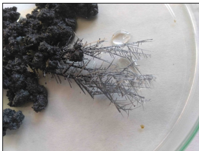
Figure 6. Photo documentation of the precipitated zinc on the cathode after the electrolysis [40]—sample B21. The appearance of cathode zinc with dendritic formations after the electrolysis has been documented. Conditions at the electrolysis are above in the text. Source: own.
