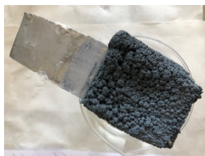
Figure 9. A photo documentation of the zinc product segregated on a stainless plate after electrolysis—sample H22. Condition at the electrolysis: cathode—stainless plate, anode—nickel plate, electrolyte—20% solution of NaOH, voltage 4 V, current 2.5 A, time 4 h and temperature 23 °C.
