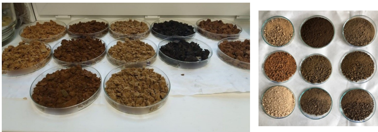
Figure 2. Preparation of samples for leaching—on the left: the delivered samples, on the right: sludge after milling and drying-up. Source: own.
