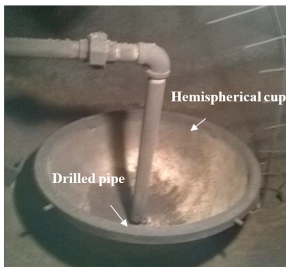
Figure 3. Drilled pipe hemispherical disperser.
