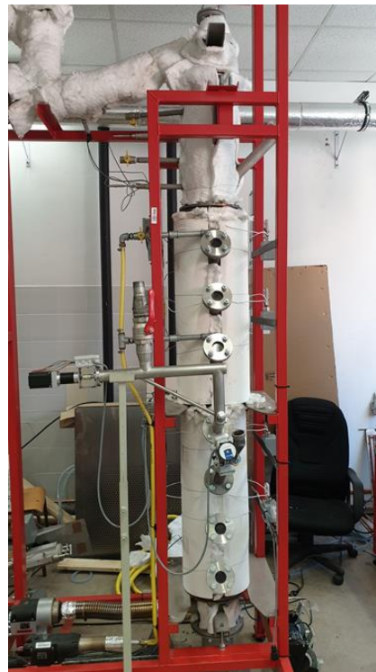
Figure 1. Scheme (A) and photo (B) of the experimental unit. Distance of temperature sensors from the grid: T1 120 mm, T2 320 mm, T3 520 mm, T4 720 mm, T5 920 mm, T6 1120 mm, T7 1320 mm, T8 1520 mm, T9 1720 mm, T10 1920mm, and T11 2120 mm.
