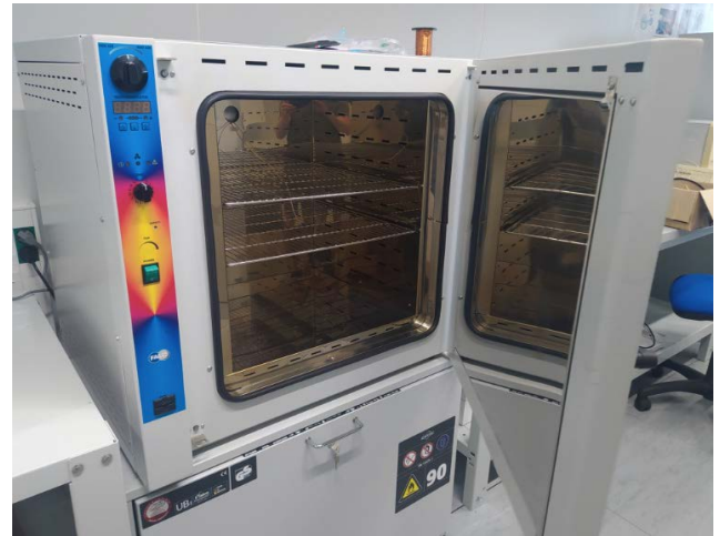
FIGURE 6. Picture of the thermal chamber serving for the sensor heating.
