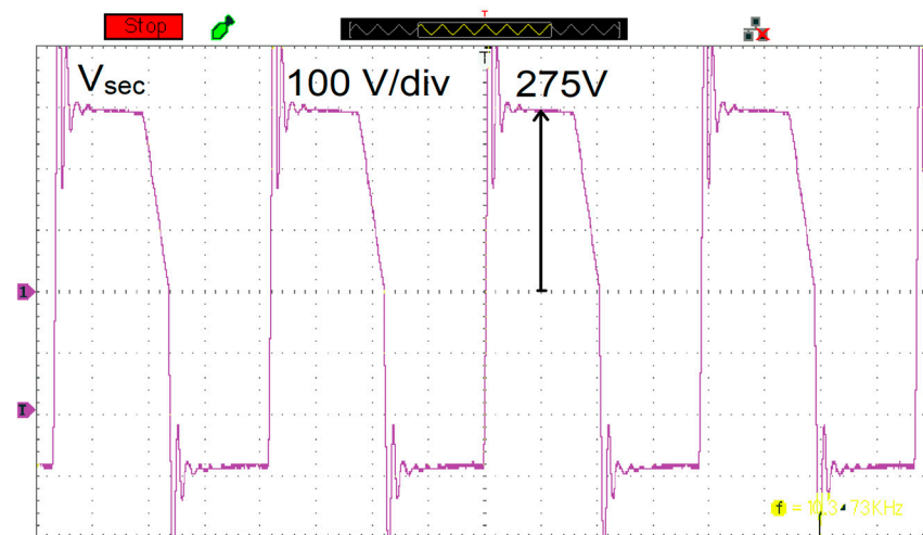
Figure 19. Secondary voltage of high-frequency transformer.
