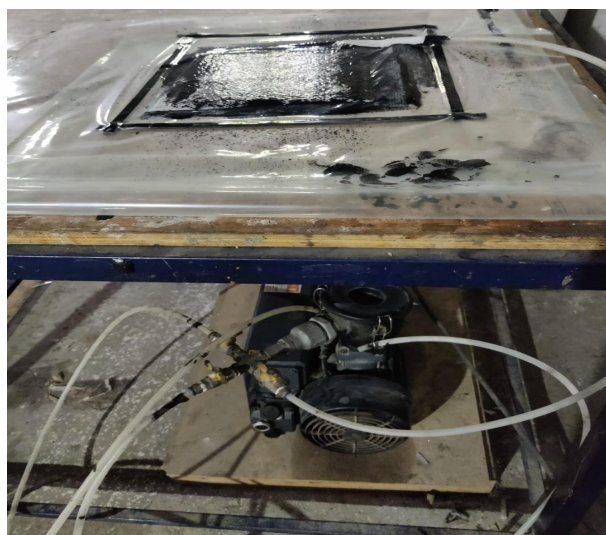
Figure 2. Vacuum infusion process.
