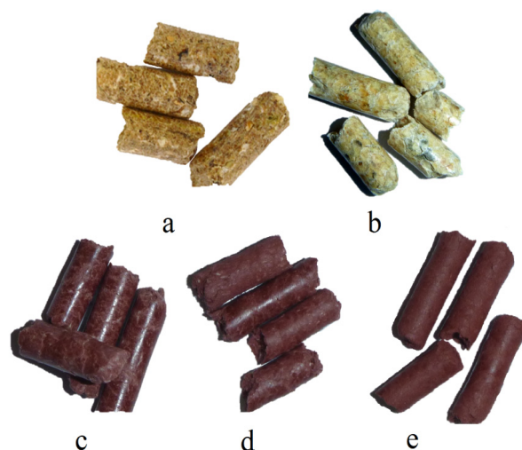
Figure 1. Examples of pellets: (a) From shredded furniture boards only; (b) From spruce wood only; (c) 5% \text{Fe}_2\text{O}_3 content; (d) 10% \text{Fe}_2\text{O}_3 content; and (e) 15% \text{Fe}_2\text{O}_3 content.
