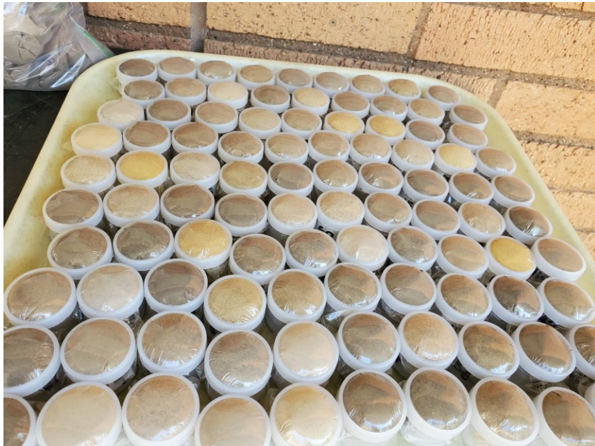
Figure 3.2: A batch of pXRF cups packed with finely ground soil ready to be scanned (Photograph by the author).
