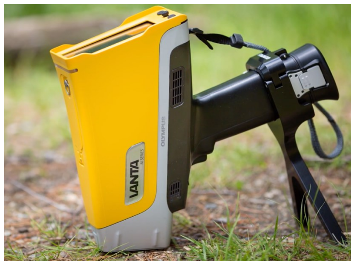
Figure 2.19: Use of a field portable pXRF mount can help address some of the error typical of in-situ analysis, like surface irregularity and sensor instability.
