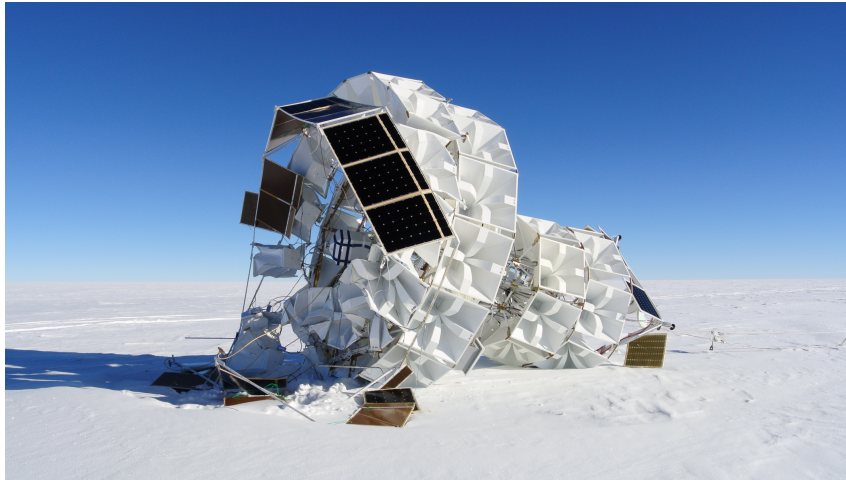
Figure 3.16: A photo of the ANITA-IV payload after crashing on the continent near the South Pole. The bottom and middle ring are “sacrificial” and were designed to crumple on landing to reduce damage to the main instrument box and payload (shown in the photo). Photo provided by Christian Miki.
