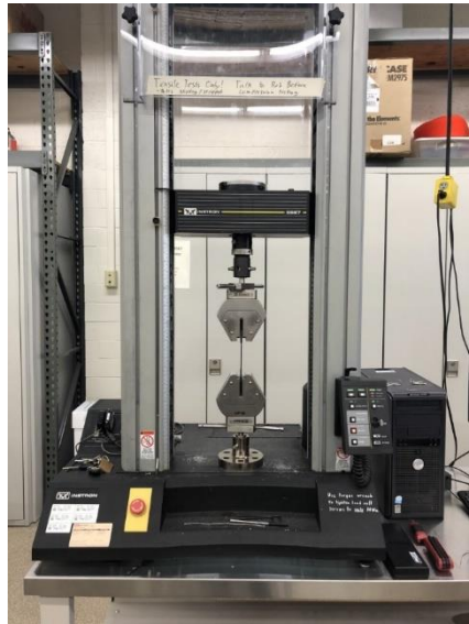
Figure 15: Instron 5567 load frame in tensile test setup
