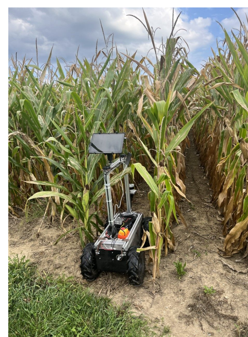
OSCAR with a LiDAR for analyzing plant physiology
