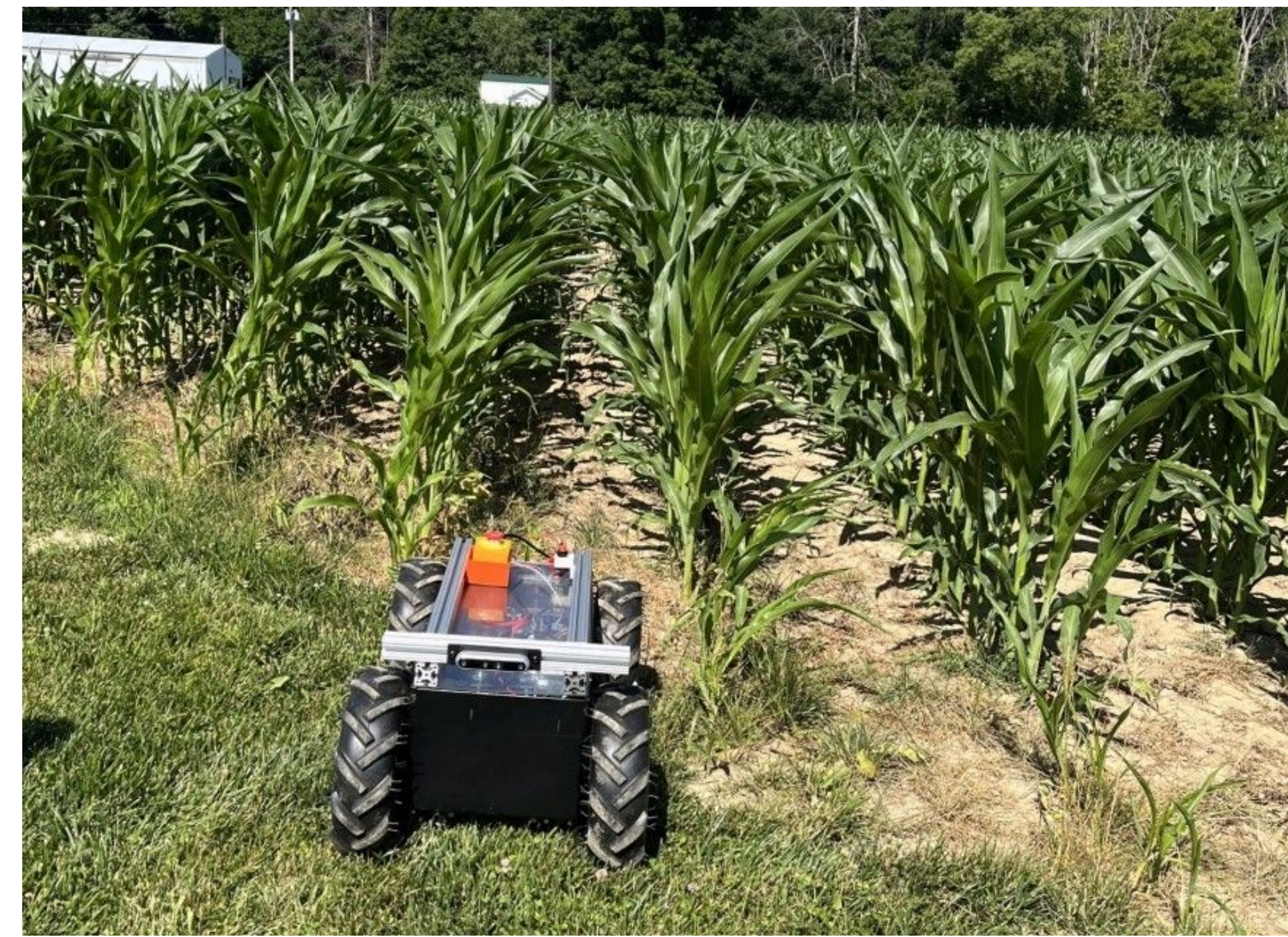
OSCAR enters, navigates and exits corn rows autonomously
