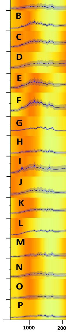
The attention map and Raman spectra for classification of several microbes and CHO cells with microbes. The bold blue line indicates average spectra (6000 scans), and the shaded area standard deviation. The heatmap (yellow-orange) indicates the importance of different segments of the spectra according to the attention map. Figure reproduced from [2].
