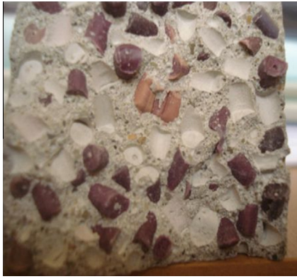
Fig. 8. The samples of self-compacting mortar with 50% content of plastic wastes.
