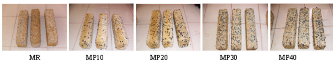
Fig. 5 State of the simples after 60 days immersion in 5 % H 2 SO 4 .
