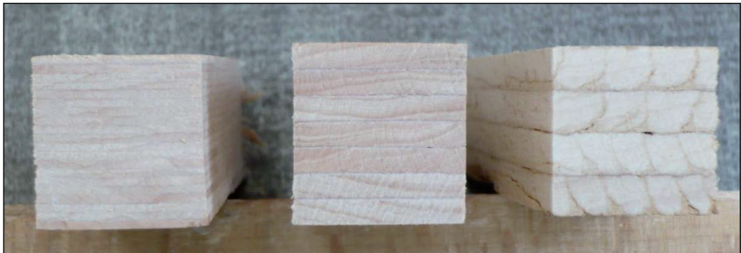
Figure 5. Cross section of the 3 kinds of sample (from the left to the right, LVL composed with 1 mm, 3 mm and 5 mm thick veneers)
