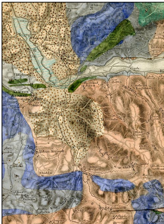
Figure 11. Detail (Newton Bushel) from old series one inch geological sheet 22, south-east Devon, surveyed 1830-31, published 1834: the first Geological Survey map to be submitted for engraving (from De la Beche's own copy, BGS Library AM 1112 S, set A).
