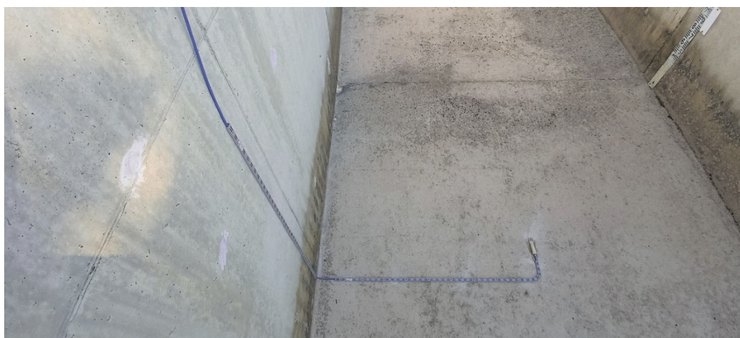
Figure 10. Picture of the sensor of the Nivus Portable Flowmeter installed in the centre of the auxiliary channel, upstream of the testing chute.
