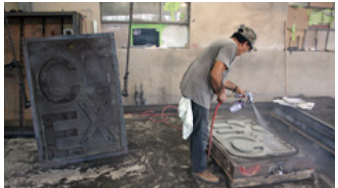
A sand-based mold is developed from a chemical-based impression.
