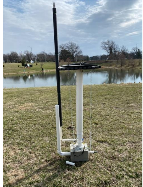
Figure SM2. Airlift pump v1 used in 2020, 2021 (left); Airlift pump v2 added in 2021 (right)
