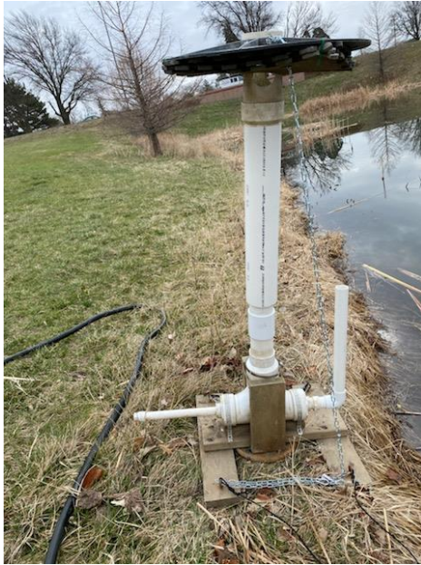
Figure SM2. Airlift pump v1 used in 2020, 2021 (left); Airlift pump v2 added in 2021 (right)
