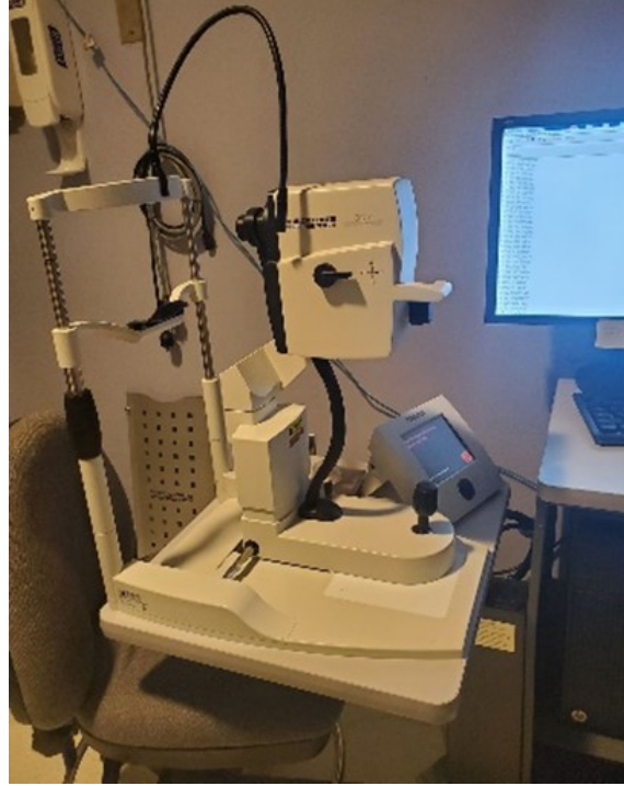
Figure 2.2: The Heidelberg Spectralis was used at each imaging session to acquire radial OCT image volumes consisting of 24 slices per volume
