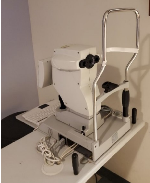
Figure 2.1: The IOL Master, a standard instrument widely used in ophthalmic clinics, was used to measure the axial length and curvature of each eye
