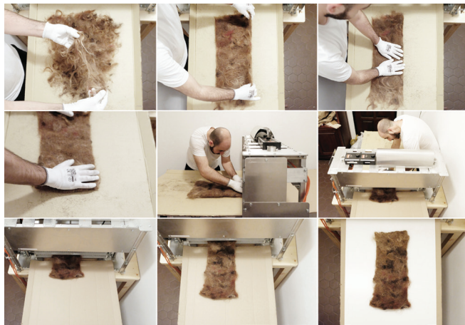
10 Hair felting machine and process.
