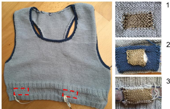
Fig. 4. Knitted garment with integrated electrodes in border (identified by square dashed lines). 1. Intarsia. 2. Double knit with cotton padding. 3. Separately knitted contacts.
