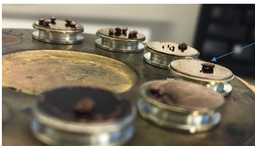
Figure 3.11: GLS-A microparticles prepared for SEM imaging
