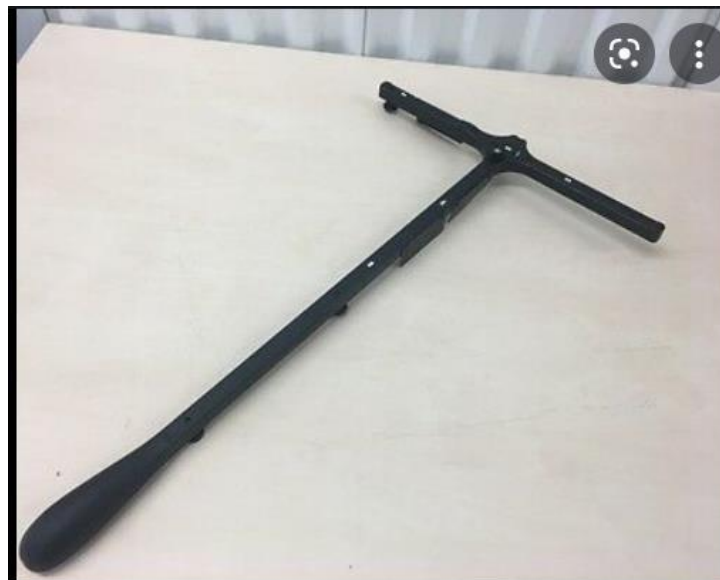
Figure 2-2 Mo-cap system calibration wand – used for spatial synchronisation
